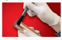
**2.** Insert the tube into the fitting until it reaches the tube stop, using a twisting action to ensure the spread of flux. Ensure the tubes are correctly lined up and adequately supported – otherwise distortion or cracking may occur when at brazing temperature.
