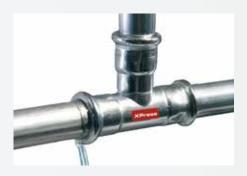
The LBP function is achieved either by a special 'O' ring or by the specific design of the fitting. This LBP function ensures that fittings, which have not been pressed, will leak during the initial pressure test. The installer can immediately see which fitting he forgot to press and correct this. Once pressed, the system is guaranteed water and air tight.
