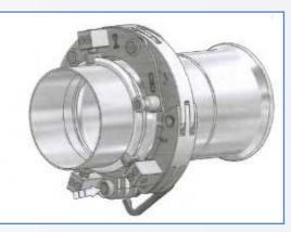
**11.** Close the collar, press the lock button, swivel the catch inwards and secure the lock.
