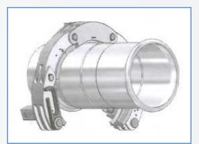
**13.** Open the lock, swivel the catch away, open the collar and remove it from the fitting.
