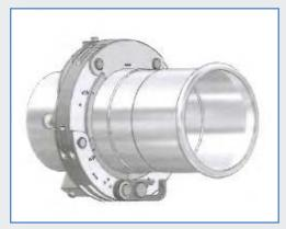
9. Perform pressing operation 1, release the catch and remove the collar. Inspect the finished joint. There will be visible witness marks from your press slings.
