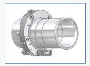
**12.** Attach the press tool to the mouth of the fitting- use the handle at the top of the press tool to open the jaws on the adapter. The claws of the adapter jaw must be firmly gripped onto the press colour.Perform pressing operation 2.
