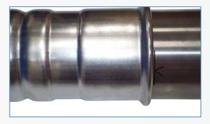
**4.** Insert the tube into the fitting until it meets the fitting stop and check that the line and 'V' marking is visible.
